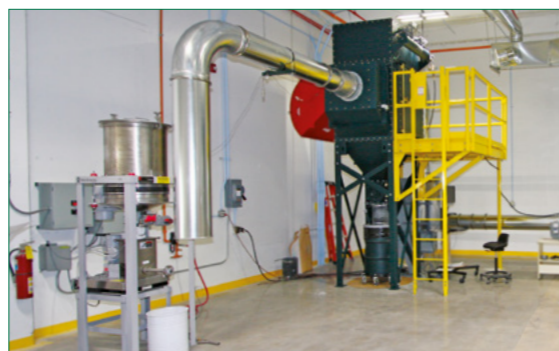
ASHRAE Standard 199 Dust Test Apparatus
